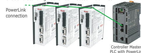
Drives control through command by master controller.
