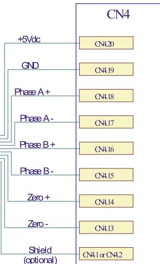
Single-Ended 5Vdc TTL/CMOS digital inputs
