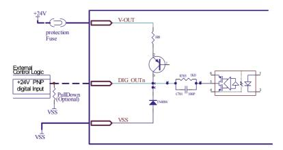
FAULT Output Logic: OK = transistor Output Closed - FAULT = transistor Output Open
