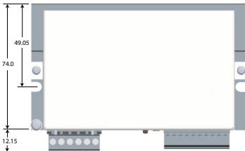
CN2: Digital inputs and output 7 position, pitch 3.81mm, PCB header connector
