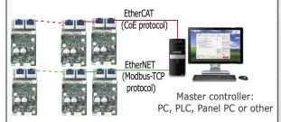
Drive control through commands by Master Controller. Suitable for multi axes systems (up to 127 drives). Built in Powerfull Motion Module functionality assures Perfect Synchronization among axes and reduces Master Controller workload
