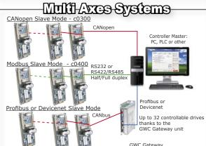
Drive control through commands by Master Controller. Suitable for multi axes systems (up to 127 drives). Built in Powerfull Motion Module functionality assures Perfect Synchronization among axes and reduces Master Controller workload
