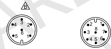
A-A' VIEW M12 MALE 6 POLES CONNECTOR MOTOR B-B' VIEW M12 MALE 8 POLES CONNECTOR ENCODER
