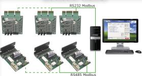
Through the serial interface is possible to control the motor position, rotation speed and control all the hardware resources of which this 'open frame' drives are equipped. For example, it is possible a check of the digital or analog I/O, or monitor the drive operating status.
